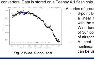
A series of ground test were performed on FINsight. - 3-point bending test on sample specimens revealed a linear relationship between load and deformation, with the slope being gauge factor. Wind tunnel test with the fin set at an angle of attack of 30° confirms measured voltage varies with square
