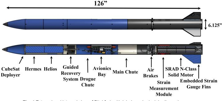
Fig. 4 External and internal view of Pitchfork with labels and principle dimensions
