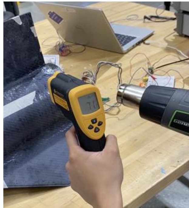
FIG 16. Thermal calibration setup
