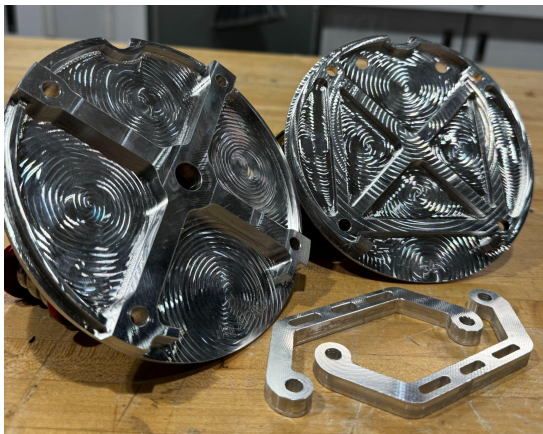
Fig. 13 Machined bulkheads and servo mounts
