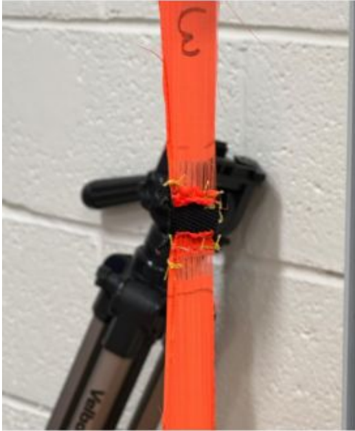
Fig. 7 Nylon Ripstop after tensile test
