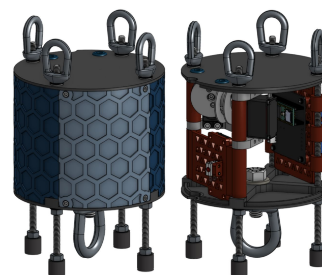
Fig. 8 Controlled Recovery Module
